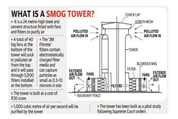
Some researchers in New Delhi have observed paradoxical phenomena near the smog towers. The air closest to the tower should be cleanest, but the device recorded the opposite in several instances.
